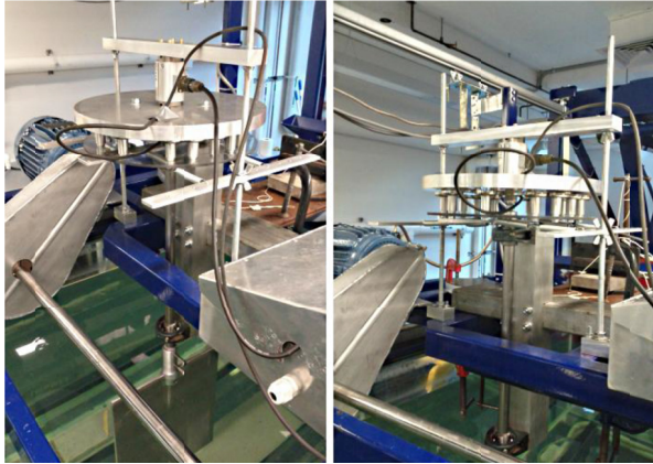
Figure 4. Experimental apparatus mounted on the towing carriage with Eddy current magnetic damper
